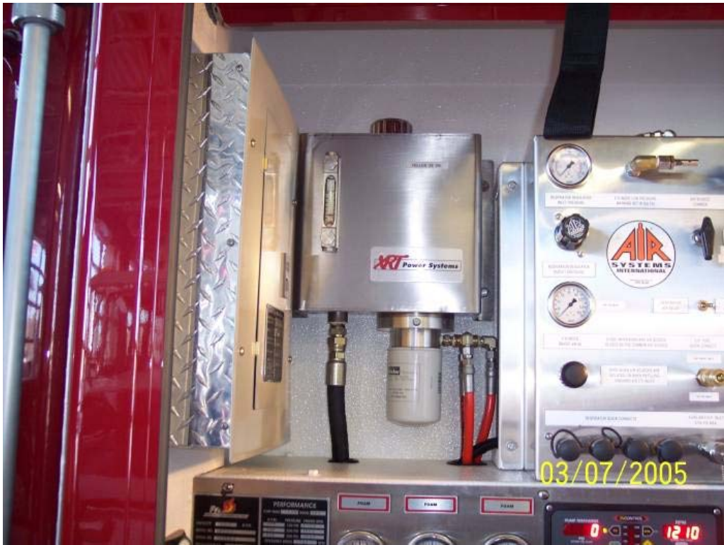
Photo 1 - Oil Reservoir Tank
