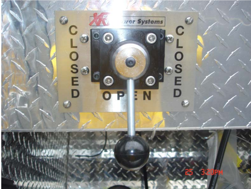
Photo 1 – Open Center Valve w/Mounting Plate
